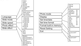
Select "SETUP" key to show setting menu,press "▲/▼" key to select setting items,press "◀/ ▶" key to adjust option,then press "ENTER" key to save the setting,press "EXIT" key to return to the first-level menu,then press "EXIT" key exit the setting menu.
